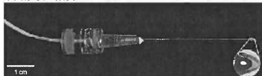
Fig. 1: Purpose-built microelectrode, with the exposed silver wire at the electrode surface (inset).
