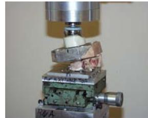
Fig 1: A intact vertebral specimen undergoing test
