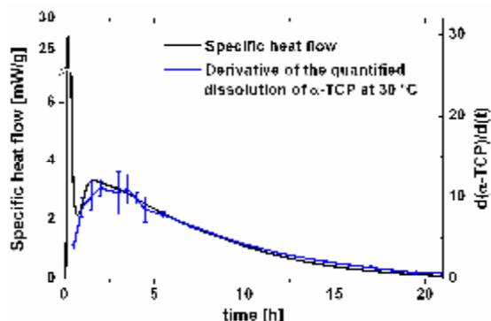
Figure 1: Derivative of the dissolved  $\alpha$ -TCP with respect to the time and the correlated specific heat
