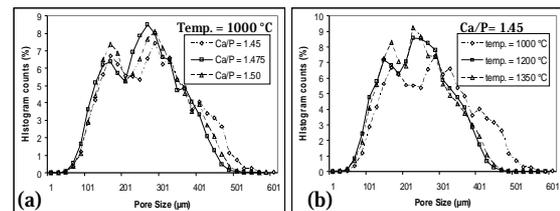
**Fig.1:** Pore size distributions as a function of (a) Ca/P molar ratio and (b) sintering temperature
