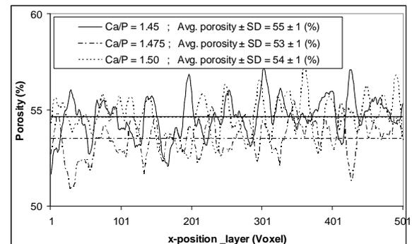
**Fig.2:** Local porosity versus  $x$ -position of layers; samples were produced at sintering tem. of 1000 °C.
