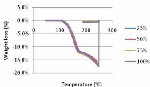
**Fig. 2** Weight loss as a function of the percentage of injected cement (on 4 ml)
