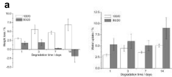
**Fig.3:** (a) Weight loss and water uptake (b) of different Heliobond®/TCP composites as a function of degradation time in simulated body fluid.
