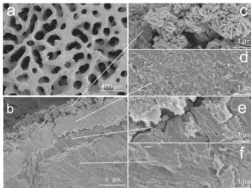
**Fig 1.** SEM Electronic micrographs of the surface structure of the CHACC cross-sections. (a) low magnification of CHACC. c-f shows sequential crosssections from b. (c) the surface crystalline HA, (d) a 5-10µm adjacent layer, (e) a junction between layers and (f) inner core structure.
