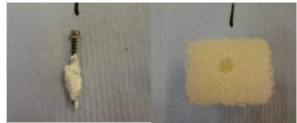
Fig. 2: (left) Screw and attached cement after pullout from sample shown (right).
