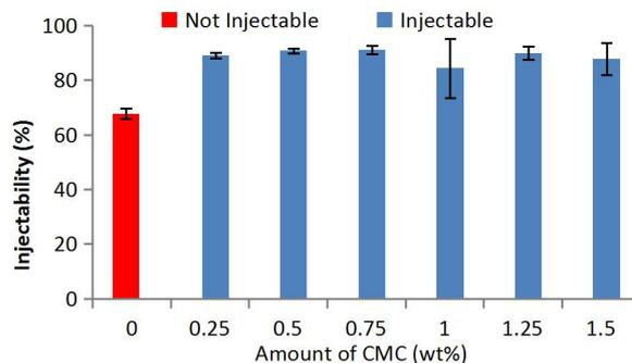
Fig. 1: Injectability of CPC containing CMC.
