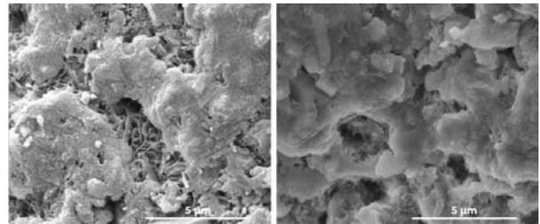
Fig. 1: SEM images of the SF CPCs (left) and tSF CPCs (right).
